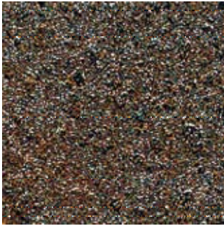
Rust Grade D
