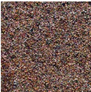
Rust Grade D
