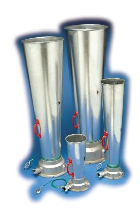
Airblast Venturi Air Blowers are a perfect solution for ventilating or extracting hazardous and explosive vapors from tanks, as well as a variety of other functions. Additionally, it can be used to cool down machinery or workers. Its function is to take high pressure air volume (from a compressor), creating a Venturi action, which results in the inhalation of large volumes of air through base. Maximum air pressure: 140 PSI.
