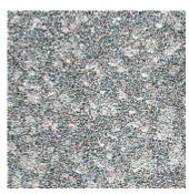
D HB2½ Rust Grade D Hydroblasted to an SA2½ equivalent
