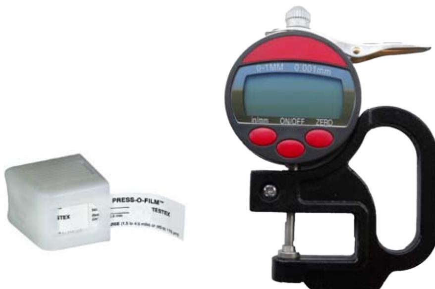
TXG-300 Testex Tape accurately reproduces the profile of the blasted surface which can be read by the TXG-320 Testex Gauge.
