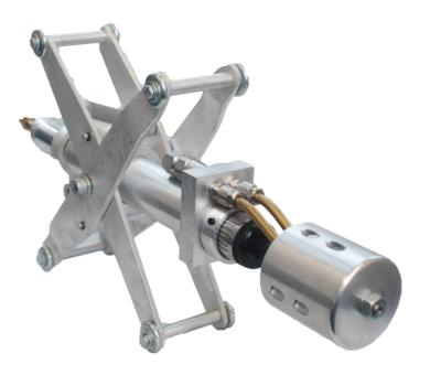
PIPECOATER-III/300 tool is designed to coat the inside of pipe or tubing ranging from 125 to 300 mm (5" - 12") ID without the need to rotate pipe or tubing and to apply an even paint film thickness throughout. Generally, any type of coating may be used in this tool that can be airless sprayed.
