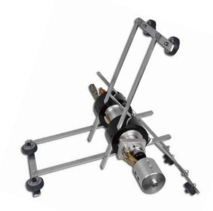
PIPECOATER-III/900 tool is designed to coat the inside of pipe or tubing ranging from 300 to 900 mm (12" - 36") ID without the need to rotate pipe or tubing and to apply an even paint film thickness throughout. Generally, any type of coating may be used in this tool that can be airless sprayed.
