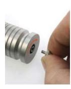
**Step 3**Turn the new tip clockwise until it's stuck.
