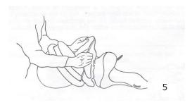
Exchanging the safety glass: Open the window frame and remove the grid and the disposable windows. The acrylate window can now be extracted out of the rubber window gasket. Take an original spare window and slide this into the window gasket.
