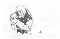
Exchanging the neck bib: The neck bib can easily be exchanged by releasing the zip. Exchanging the cape: The bib/cape can be exchanged by shoving away the rubber helmet cover partly (fig. 5).
