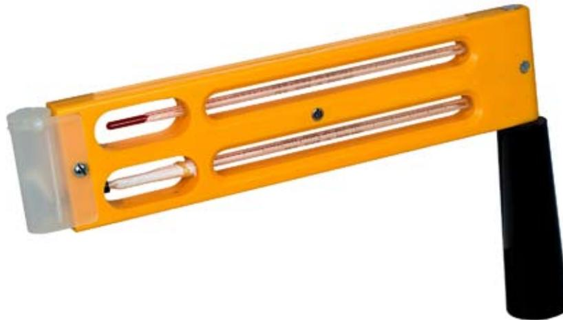
The WHM-130 can be used to calculate the prevailing dew point temperature quickly, easily, and economically in combination with a dew point calculation table.
