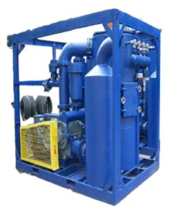
AIRBLAST ABVR series vacuum recovery system is designed to recover spent dry recyclable abrasives from a blasting area into a silo for subsequent return to the blast cleaning equipment or, in the case of expendable abrasives, for disposal into a waste hopper.
