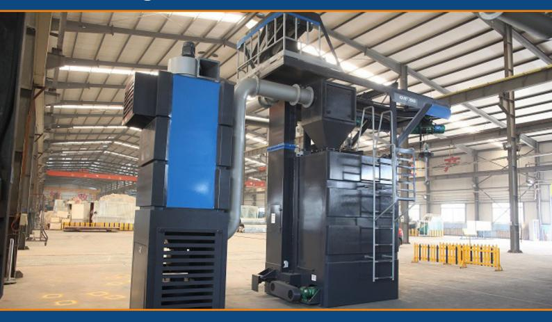
Shot Blasting Machines utilize multiple spinning blast wheels as opposed to air pressure to propel abrasive onto the substrate. As the spinning blast wheels are fixed in place each machine is designed to blast a certain substrate shape in the optimum way. The production characteristics of each wheel blast machine is determined by the quantity, power, and size of the spinning blast wheels.
